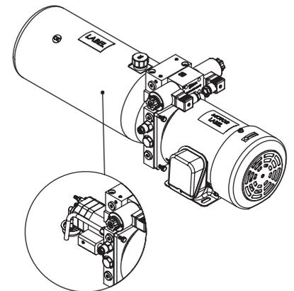
The W83A series power pack is designed for applications that need high pressure and larger flow, but use a low-power A.C. motor. The power pack uses a special manifold (W800553). All screw-in cartridge valves have been designed to be adjusted easily to service the power pack quickly. They still have the same dimensions and functions as the standard manifold (W800532).
